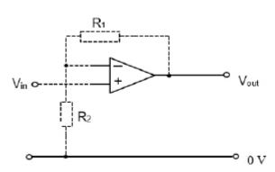
Correct configuration of  $R_1$  and  $R_2$
