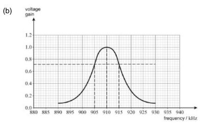
General shape around  $f_0$  and to max of 1.0 on relative voltage gain axis
